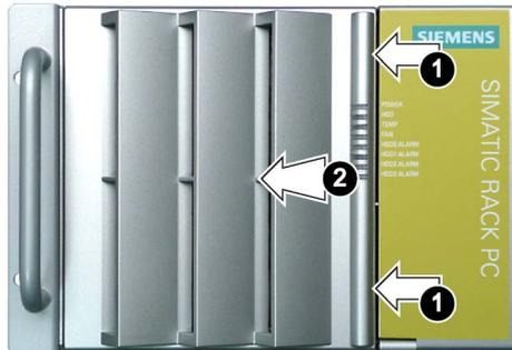
1. Press the marked at the same time to release the fan cover.
