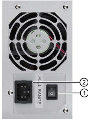
1. Make sure that the on-off switch ① is in the '0' (off) position.
