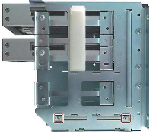
The figure below shows the positions of the screws on the right side of the drive cage.
