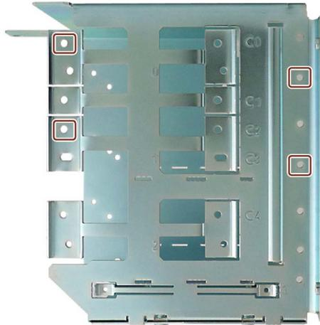
The figure below shows the possible positions of the screws on the right side of the drive cage.
