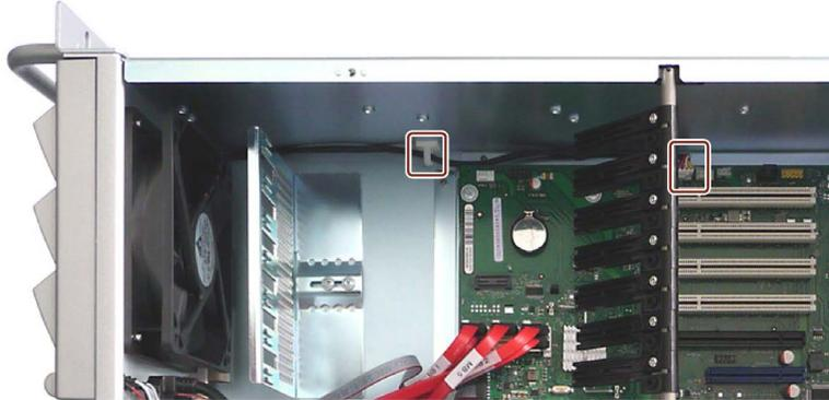
2. Remove the screws highlighted in the following figure.
