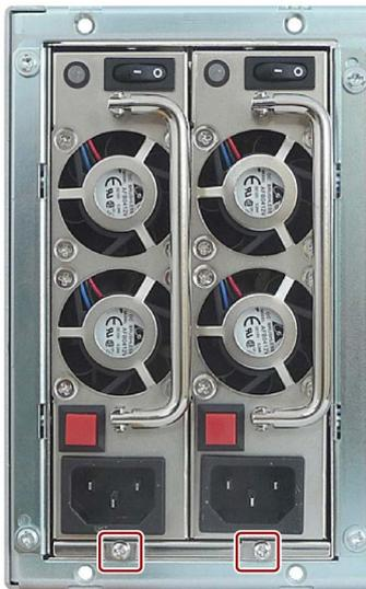
1. Remove the screws that are marked in the figure below.
