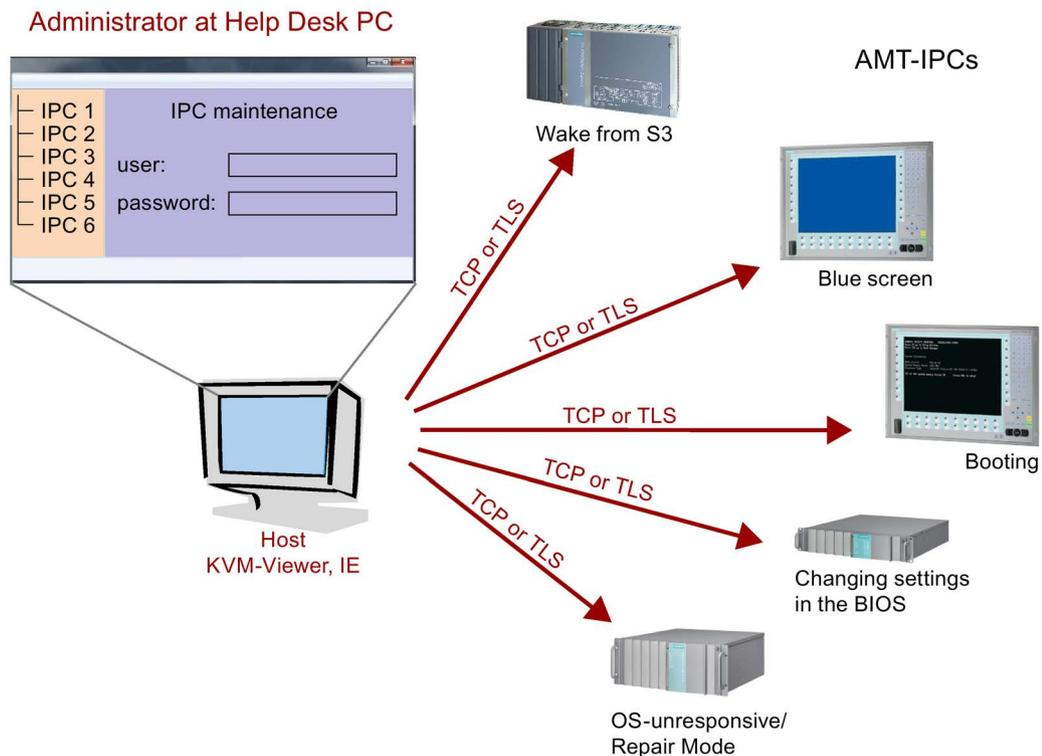
From a SIMATIC IPC which does not have Intel AMT functions, you can access networked SIMATIC IPCs with Intel AMT using the SIMATIC IPC Remote Manager and/or a web browser.
