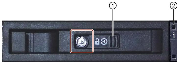
4. Open the lock with the appropriate key.
