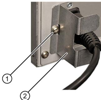
1. Remove the retaining screw ①.
