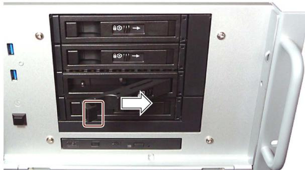
4. Now grip the handle to the right of the notch from where it was pulled out, and pull the tray all the way out of the removable drive bay.
