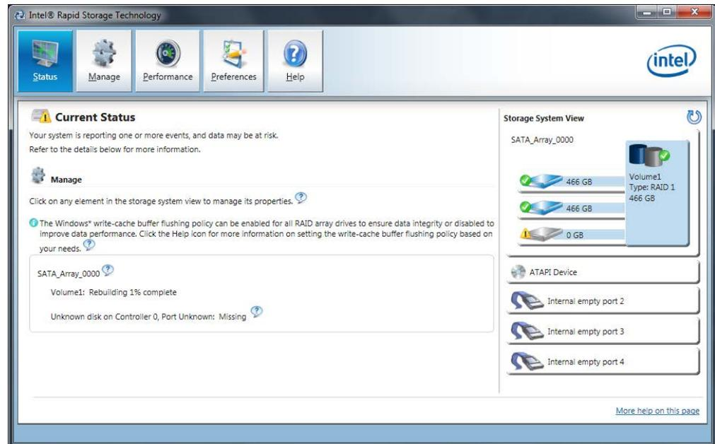
If you shut down and restart the system without installing a functioning new hard disk, "unused" is displayed for the corresponding SATA port. You can install the functioning hard disk while the system is running. The new hard disk is then assigned to a SATA port and is integrated into the RAID system.
