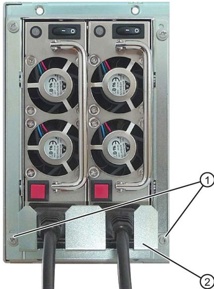
1. Remove the retaining screws ①.
