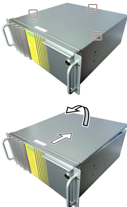
1. Remove the highlighted retaining screws.
