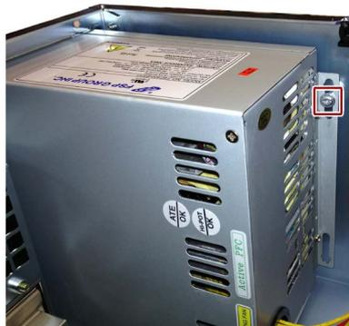
4. Remove the four fixing screws that are marked in the figure below.
