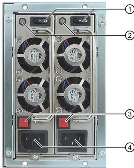
1. Make sure that the on/off switch ① is in the '0' position.
