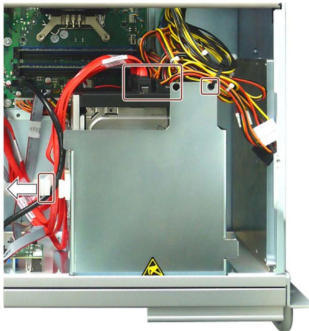
3. Hold the drive cage at the marked areas, push it in the direction of the arrow, then lift the drive cage completely out of the device.
