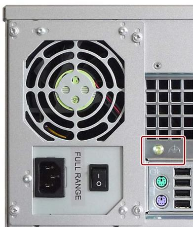
1. Connect the identified equipotential bonding connection to the protective conductor of the control cabinet in which the device is installed.
