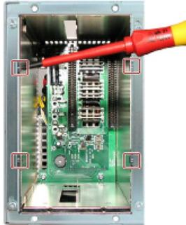
1. Remove the cable ties securing the power cables in the enclosure.
