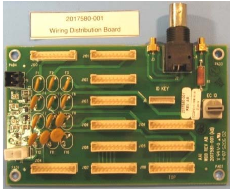
Figure 2-39: Wiring Distribution Board
