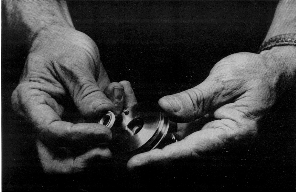
Figure 4-34: Installing Bal-Seal (20) in Piston Groove (18)
