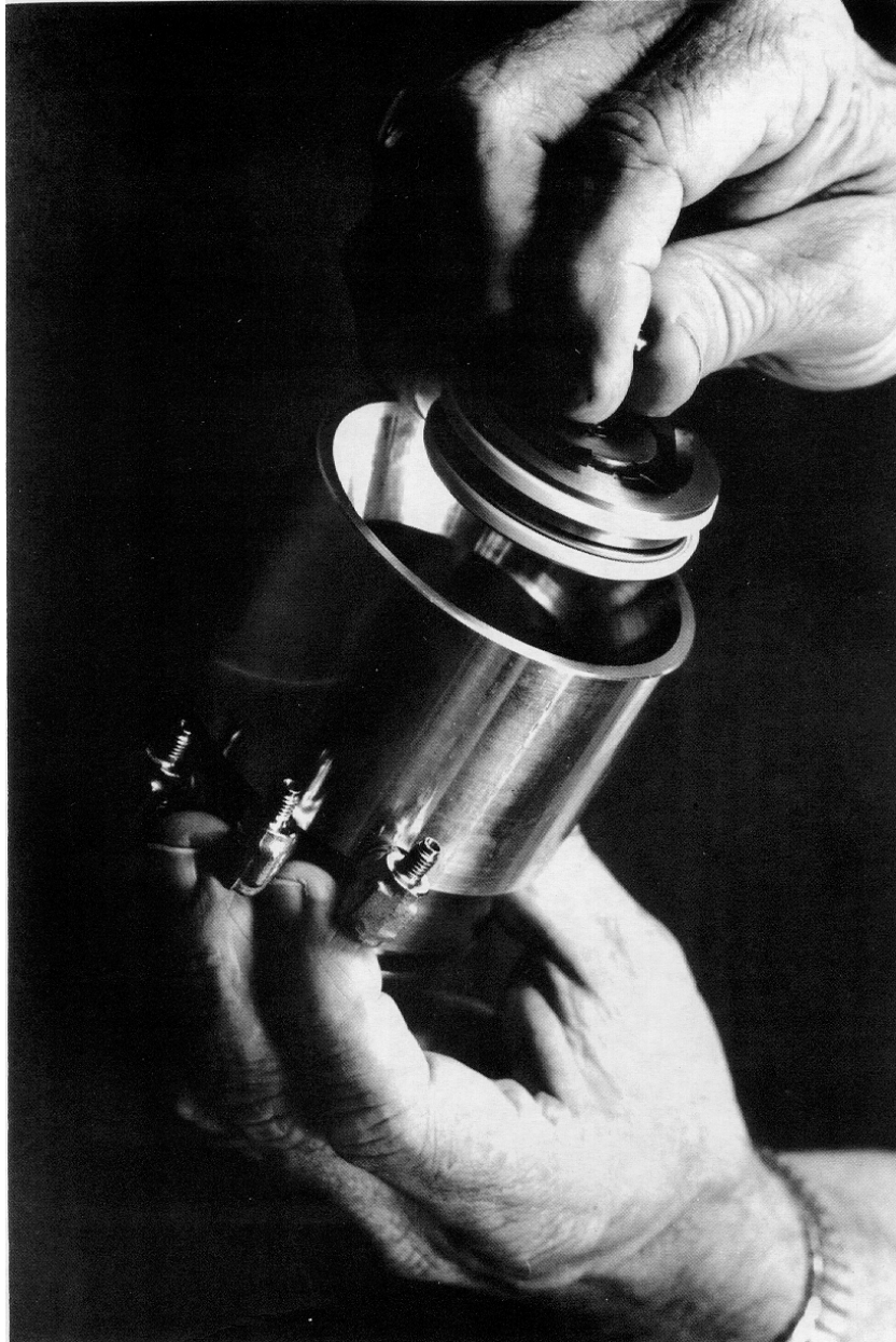
Figure 4-36: Inserting Piston Assembly (15 and 18) into Base (16)
