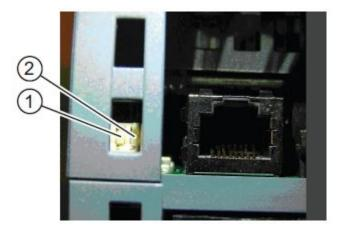
DIP-switch 1 has currently no function. Switch number 2 needs to be in the lower position for the Stand-Alone-Mode without PLC.
